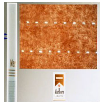
Ventilation holes in the filter paper around Marlboro Lights cigarettes.
